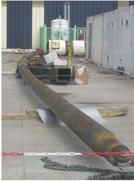
Figure 1: Rosa Pipe-in-pipe bent to a radius of 29 m. The test piece is instrumented with strain gauges.
