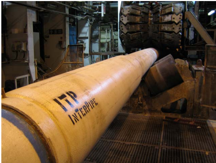
Fig 6: ITP field joint sleeve on the firing line
